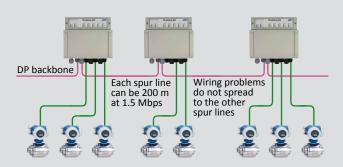
Example of dynamic spur lines to instruments. The devices can be added and removed during operation.
