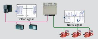
Example of the barrier function of the ProfiHub. Noise and EMC disturbances will not affect the backbone or the other channels.
